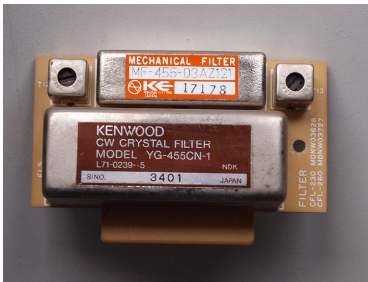
Optional filter board for NRD 515 with 2,4 kHz mechanical Filter and a NDK crystal filter (same size as YF-series)
